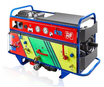
The two mixing systems are distinct, this allows simultaneous dispensing and, either only at high or only at medium pressure of the foamed mixture ensuring maximum versatility, the use of the mixing system(s) allows not only the use of foaming agents but also of mixable products for various types of fire prevention, reclamation, disinfection, disinfestation treatments, etc.
