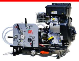
an effective and pushed atomization. The motor pump is equipped with an automatic acceleration system which automatically accelerates the engine when the water/foam lance is opened and decelerates when the lance is closed. This system quarantees lower fuel consumption, safequarding the environment, and the motor pump can be used by a single operator.
